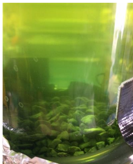
Flooded column leach setup P 100 5.6mm High Grade lumps in heated 20% H_2SO_4 solution at 20% pulp density and high upward flow rates
