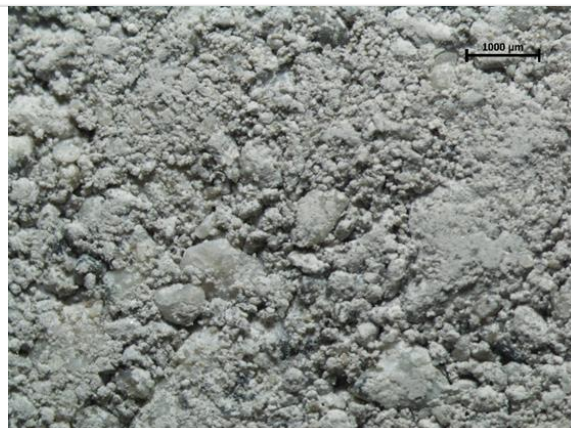
Leach Residue Vat Leach Test of 3.35mm lump 20% H 2 SO 4 70°C after 10 days
