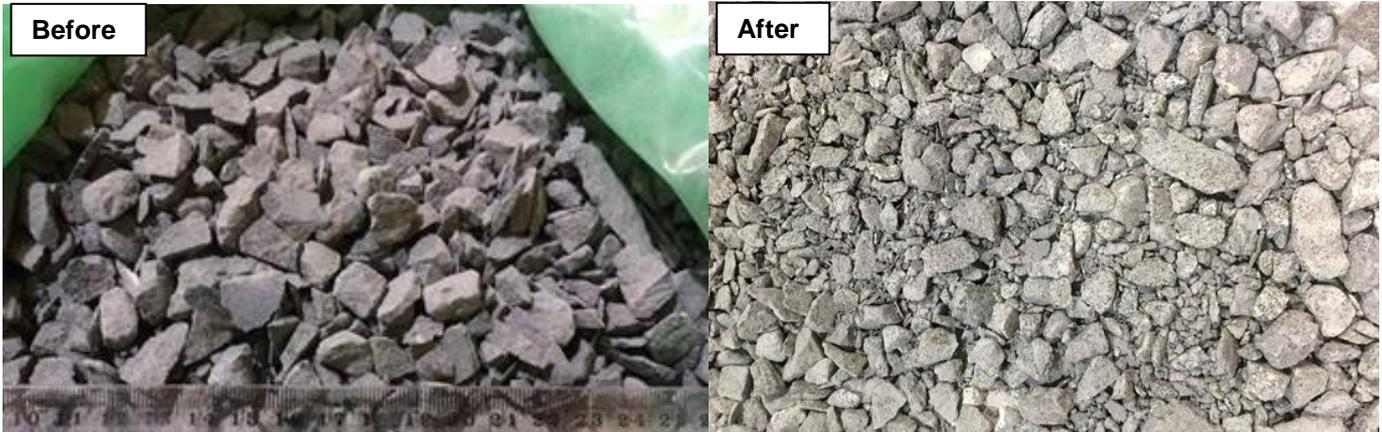
The leach plots of V and Ti extractions vs time still have positive slopes indicating the leaching process had not completed after 45 days (see graph below for 5.6mm lump size result). Most of the Al and Mg extraction occurs early in the leach profile suggesting that the more soluble alteration and rock rocking minerals dissolve more readily then show very little extra extraction.
